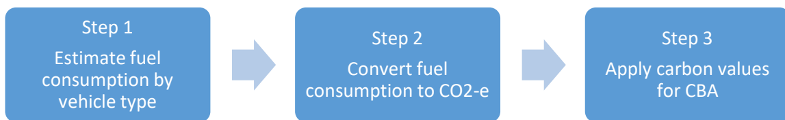
Figure 1: Steps of measuring carbons from transport operations
