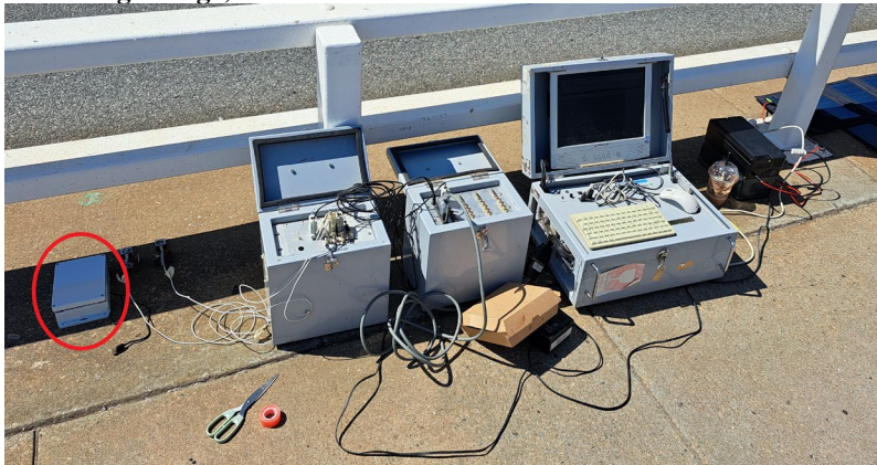
Figure 3: The IoT prototype sensor (circled in red) and the wired accelerometers set up for roadside testing at Stirling Bridge, WA
