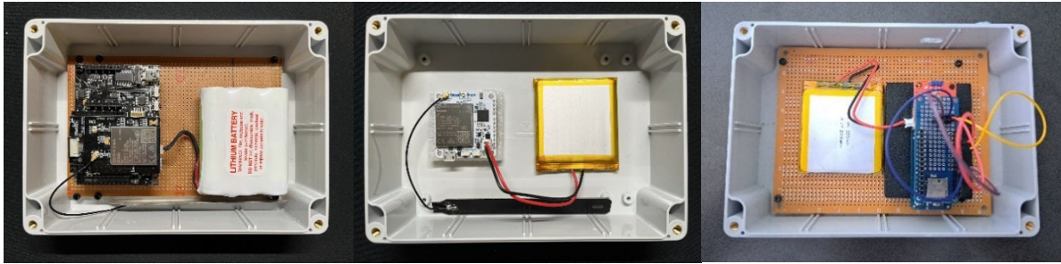
Figure 2: From left to right, Libelium Waspote, RAKwireless WisTrio RAK5010 and Arduino MKR NB 1500
