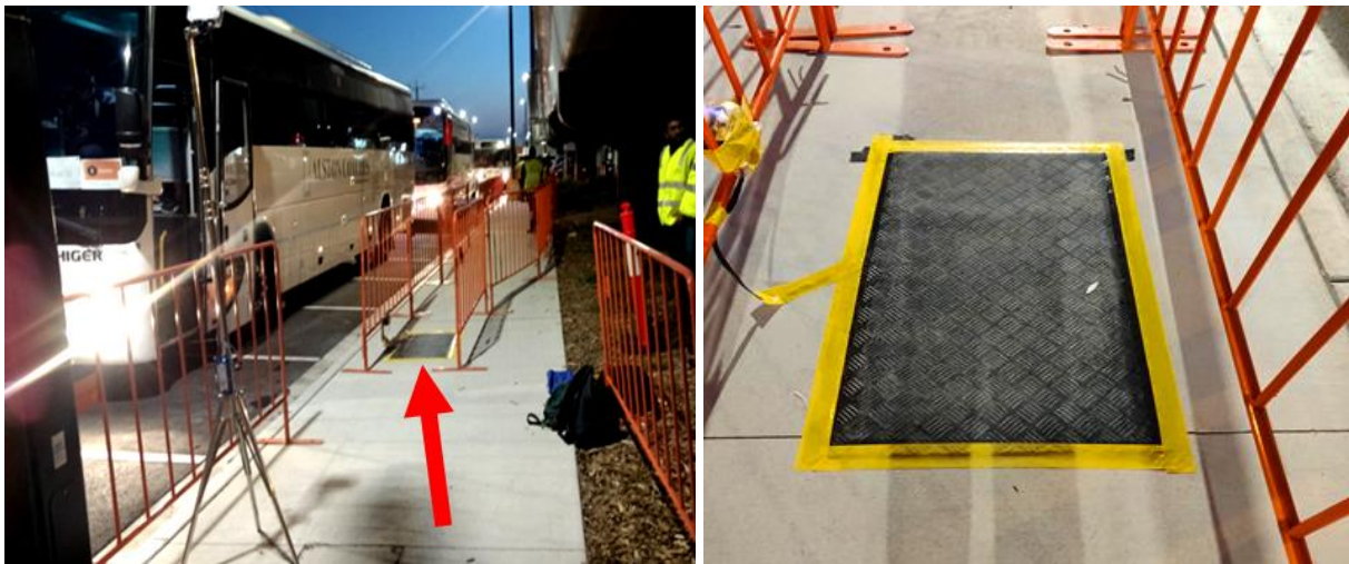
Figure 1: The Sensor Mat prototype used for passenger counting
