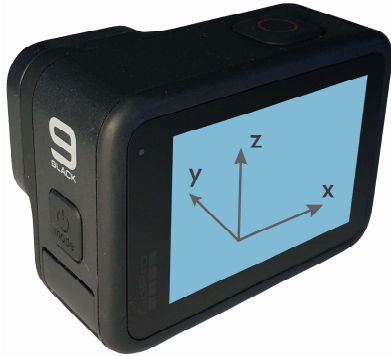
Figure 1: Arrangement of the axes on the GoPro
