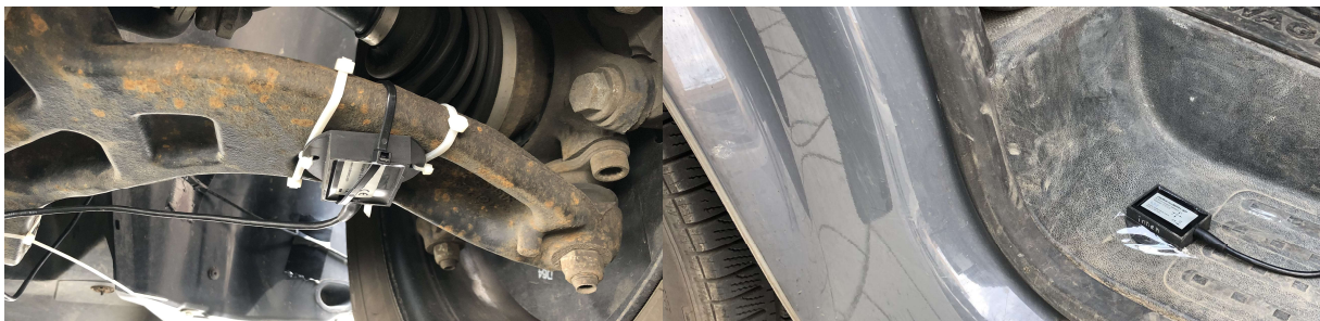
Figure 3: Measurement setup with two accelerometers
