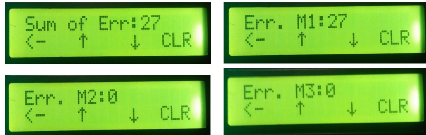
Figure 10: Lost data packets are represented by “error” (Err.)
