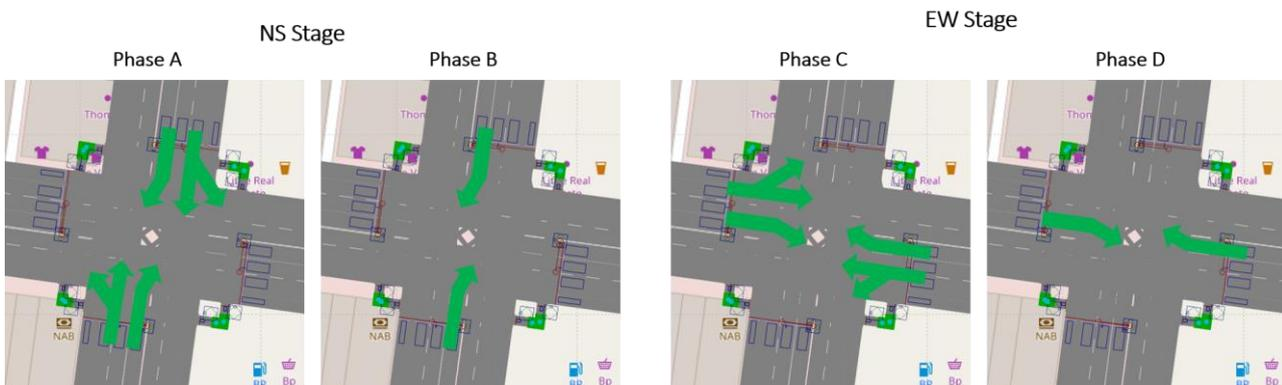
Figure 2: traffic signal phases of simulated intersection
