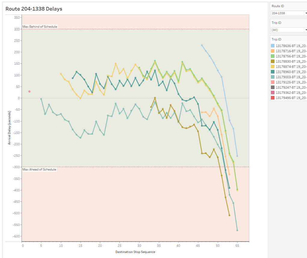
Figure 8: Arrival delays at sequence of stops along a transit route (for a number of trips).
