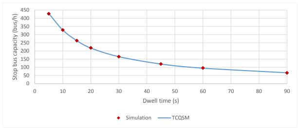
Figure 2: Bus capacity of testbed bus stop versus dwell time (Case 1 Away from Influence of Signalized Intersection)
