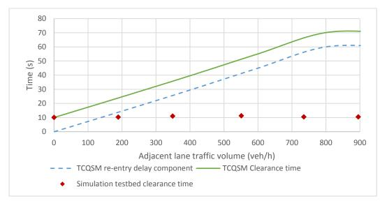
Figure 5: Delay components of clearance time versus adjacent lane volume for a bus stop upstream of a signalized intersection
