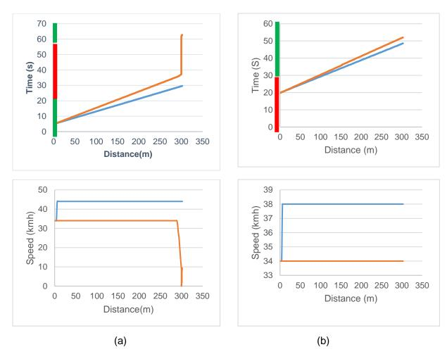
Figure 3: Manoeuvring of a control vehicle with the speed control algorithm (Blue colour) and without the control algorithm (Orange colour) (a) A vehicle approach the intersection during at the beginning of the green signal (b) A vehicle approach the intersection at the end of the red signal
