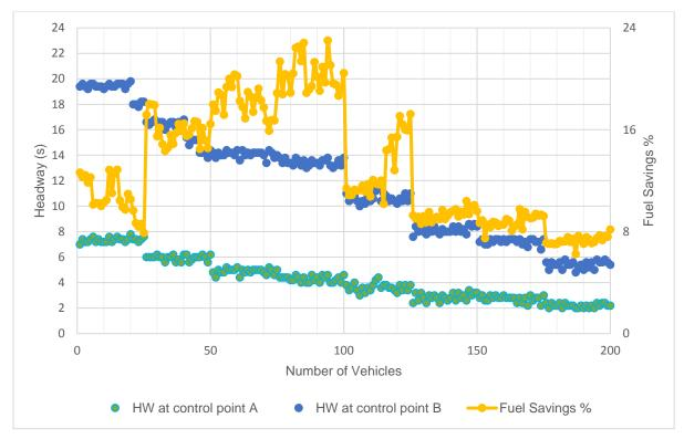
Figure 6: Relationship between headway and fuel savings %
