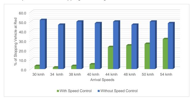
3.2.3 Impact on Vehicle Stopping at Red Signal
