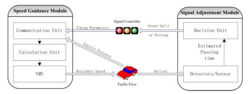
Figure 1: DSDS framework logical structure (Chen et al., 2011)
