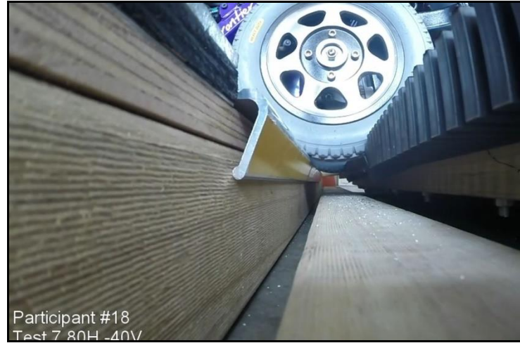
Fig 19: Image of gap filler deflecting under load (below right)
