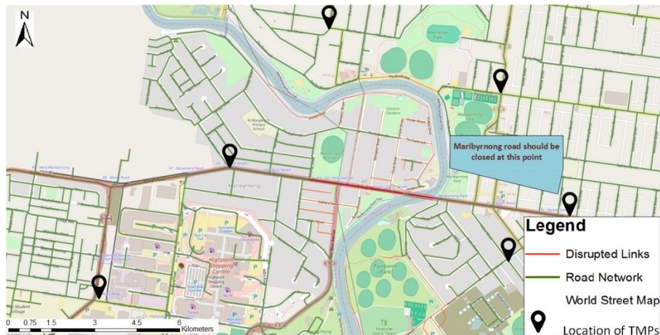
Figure 7: Proposed locations for TMP on the road network (roads in red are disrupted)
