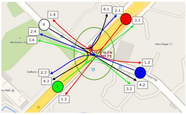
Figure 9: Schematic of Cadbury Junction with Section numbers (circled) and turning moments (by colour of origin section).
