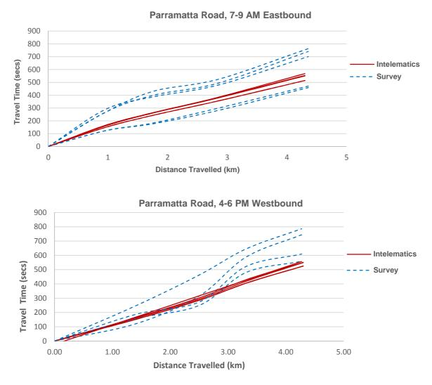
Figure 2: Intelematics and floating car survey travel time comparison, Parramatta Road at West Street to Cleveland St to Botany Rd and O'Riordan Street
