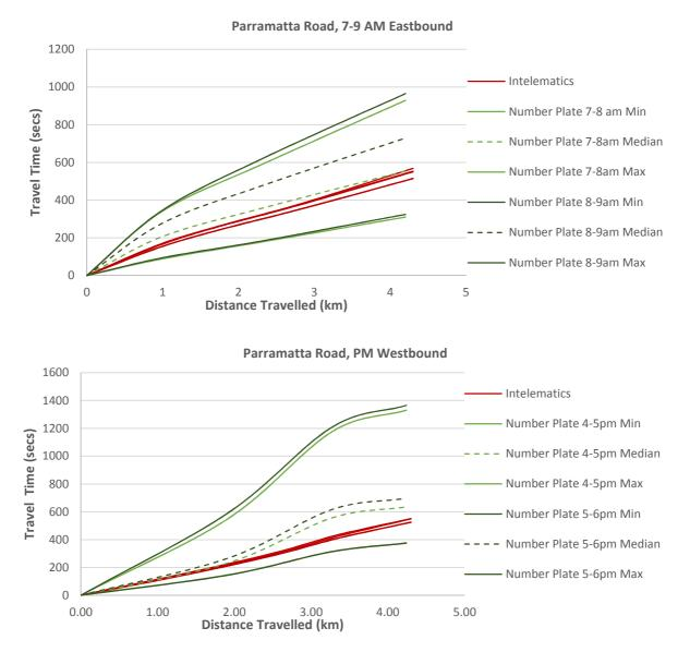
Figure 4: Intelematics and Number Plate survey travel time comparison, Parramatta Road at West Street to Cleveland St to Botany Rd and O'Riordan Street
