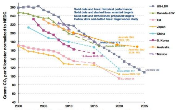
Figure 5: Comparison of new passenger vehicle fleet average emissions, actual and forescast (ICCT 2011)
