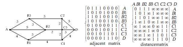
A simple network is shown in figure 1. The adjacency matrix and the distance matrix are obtained based on the relationship of distance and the vertex. It is easy to get the shortest distance from vertex A to vertex D based on the Dijkstra algorithm (Fuhao ZHANG, Ageng QIU, Qingyuan LI, 2007).
