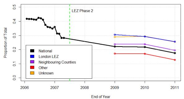
Figure 8: Proportion of non-compliant rigid vehicles in the LEZ
