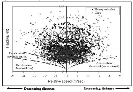
Figure 7. Observed space headway as a function of relative speed.
