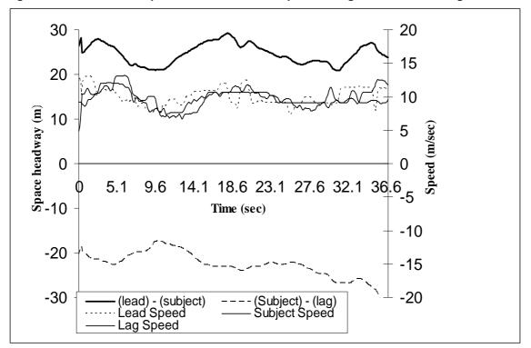
Figure 5. Relative vehicle positions and vehicles speed during truck-car following.
