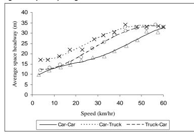
Figure 3. Speed-time headway observed in real traffic.
