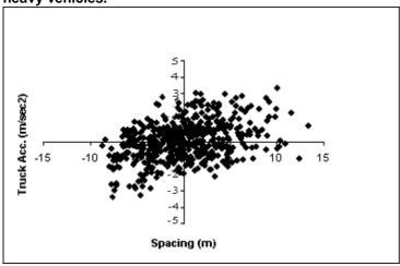
Figure 8. Heavy vehicles acceleration rate vs. spacing between the freeway leader vehicles and heavy vehicles.
