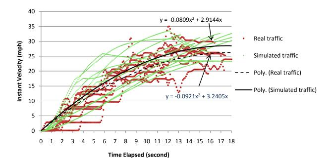
Figure 5: Real discharge velocity and the simulated discharge velocity (after calibration)
