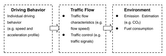
Generally, there are two approaches to assess the impacts of driving behaviors; they are field tests and traffic simulations. When considering the impacts on traffic flow, traffic simulations have obvious advantages over field tests. Traffic simulations are able to replicate various traffic conditions in computers, while the field measurements will be labor-intense and time-consuming in testing different scenarios. In addition, a traffic simulation can generate
