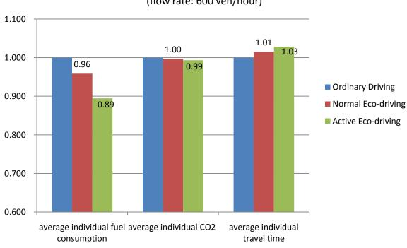
**Different Acceleration Rate** (flow rate: 600 veh/hour)
