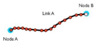
Links represent the centreline of the road's CrossSection (introduced in Level 2), so the geometry described in Level 1 has to represent the centreline of the full cross-section – not the road only. WayPoints, are describes, such as Nodes, in 3-dimensional space by their coordinates (i.e., x, y, z) based on the World Geodetic System WGS84, and the new radius of the link.
