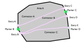
Connectors do not hold information on traffic rules or behaviour, but plainly describe the movement of a vehicle from an entry to an exit.
