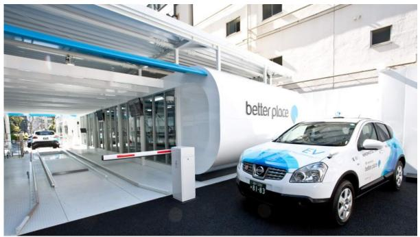
Figure 1: The battery switch station in Roppongi Hills, Tokyo, used in a 2010 electric taxi trial run by Better Place
