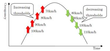
• Step two: the logic of determining new speed limit can be retrieved from the speedflow relationship curve (see Figure 4). According to the speed-flow curve, different speed limits have different maximum stable flow rates. Therefore, the logic of speed limit selection is stated as follows:
