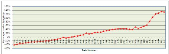
Figure 11: Percentage difference in calibrated versus uncalibrated load
