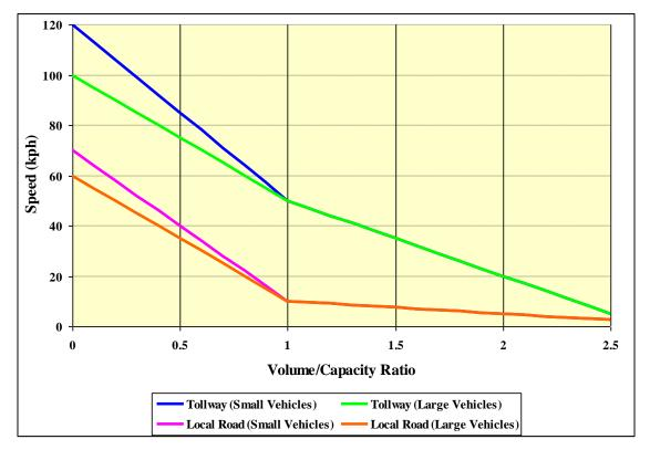
Figure A4.1:Speed-Flow Curves by Link Type and Vehicle Type
