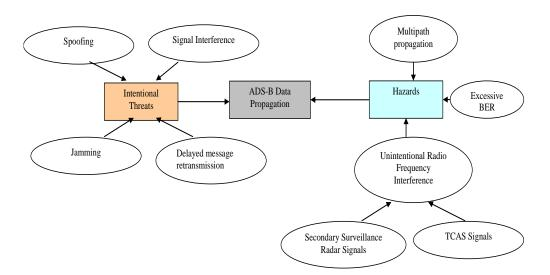
Figure 6: ADS-B Propagation path Threats and Hazards
