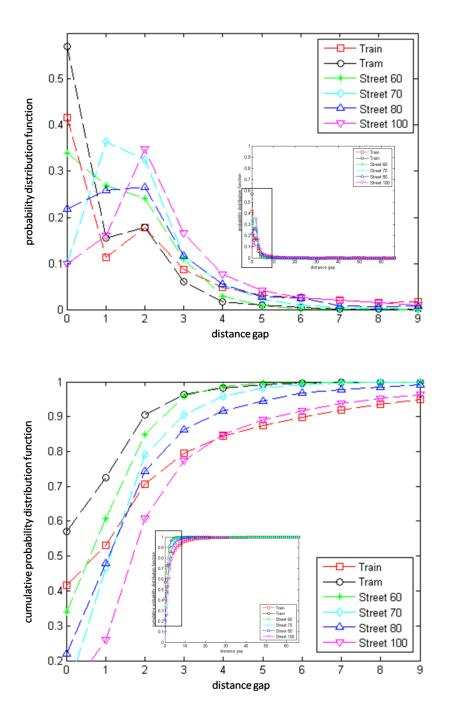
Figure 4: Distance gap – probability distribution function (top) and cumulative distribution (bottom)
