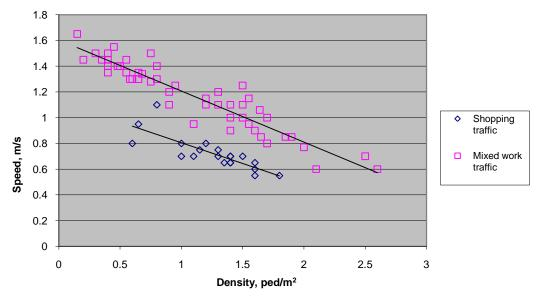
Figure 1. Speed-density plot of shopping and work traffic (Source: Oeding, 1963)
