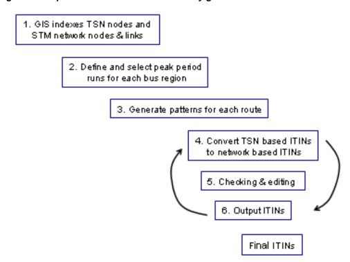
In the first phase the STM network nodes and links are extracted from Emme, and then GIS is used to create a corresponding table of the stop nodes, STM network nodes and STM network links. The links are used to reduce node misallocation.
