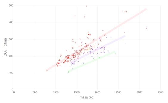
Figure 2: CO<sub>2</sub> emission rates and vehicle mass for new vehicles in Australia, 2008
