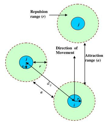
Figure 2: Components of the interactive forces
