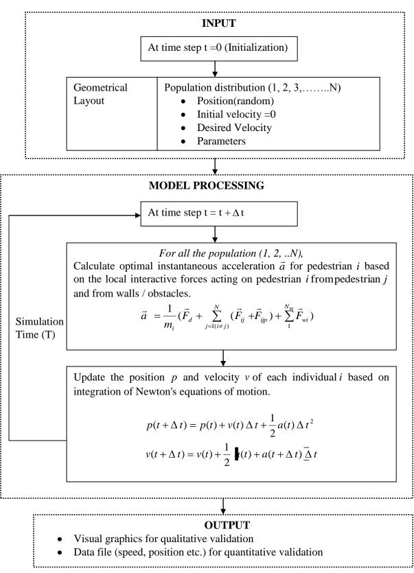
Figure 1: Flow chart of simulation program
