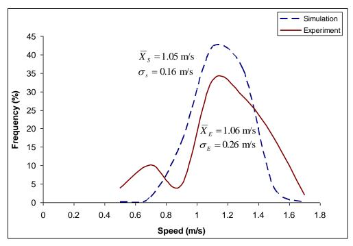
Figure 4: Comparison of speed data distribution from simulation with experiment for unidirectional traffic
