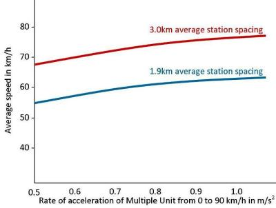
Figure 2 Average train journey speeds achievable with different station spacings (adapted from the ART report)
