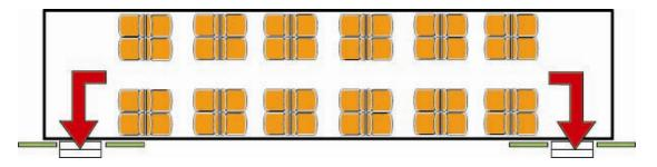
Above:- Diagram of an end vestibule entranceways (EVE) with steps and manual doors (Morlok & Nitzberg 2004).
