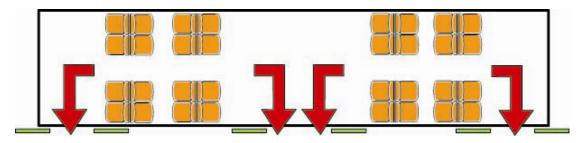
Above: - Diagram of a short dwell entranceway (SDE) level with platform and automatic doors (Morlok & Nitzberg 2004).
