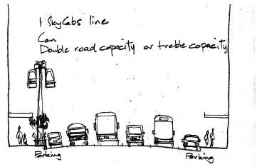
A single two-way SkyCabs line with eight-seater cabs and frequency of up to six seconds between vehicles gives a capacity of 4800 passengers per hour. Therefore the single two-way line can match the capacity of a four lane motorway and, with the additional eight standing passengers, i.e. over 9000 pphr, that of an eight lane motorway.
