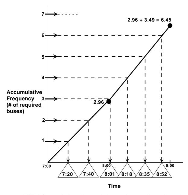
FIGURE 2 Determination of the example departure times (at A) for evenly spaced headways with a smoothing process between time periods
