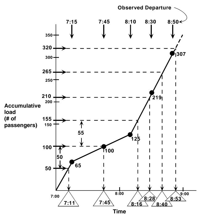
**FIGURE 3** Determination of the example departure times (at A) with even loads at the hourly maximum load point
