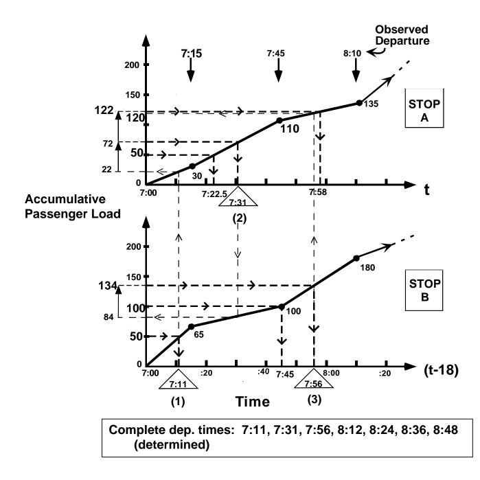
FIGURE 4 Determination of the first three departure times (at A) considering even loads at the individual bus maximum load point
