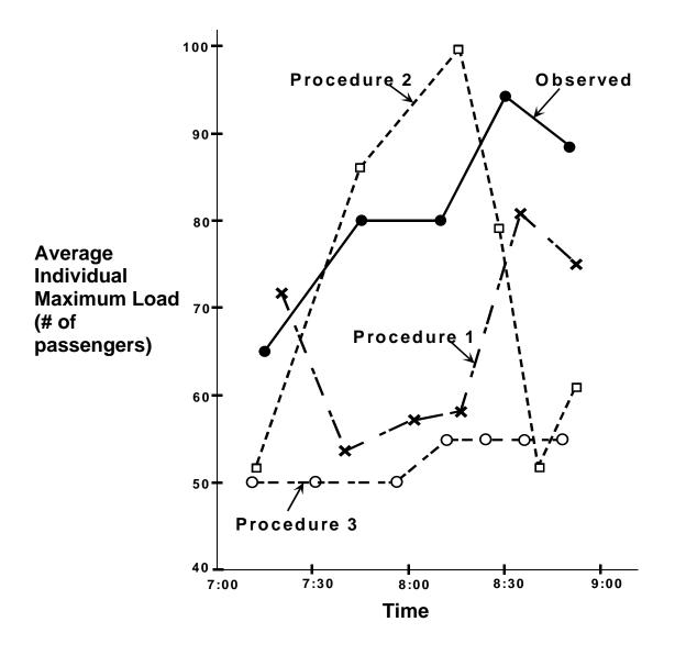
**FIGURE 5** The example departure times and average maximum loads on individual buses as observed and obtained by the three procedures
