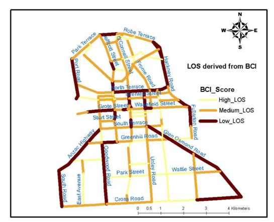
Figure 1 – Bicycle Level of Service derived using Bicycle Compatibility Indices
