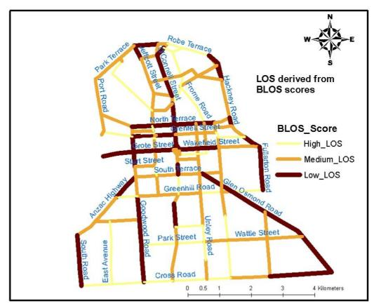
Figure 2 - Bicycle Level of Service derived using BLOS scores
