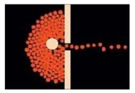
Figure 1 – Simulation showing flow in the presence of a column at the exit (Helbing et al., 2002)
