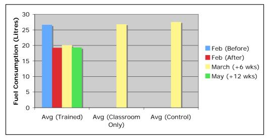
Figure 3 – Field trail results: Fuel consumption
