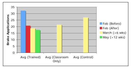
Figure 6 – Field trial results: Number of brake applications
