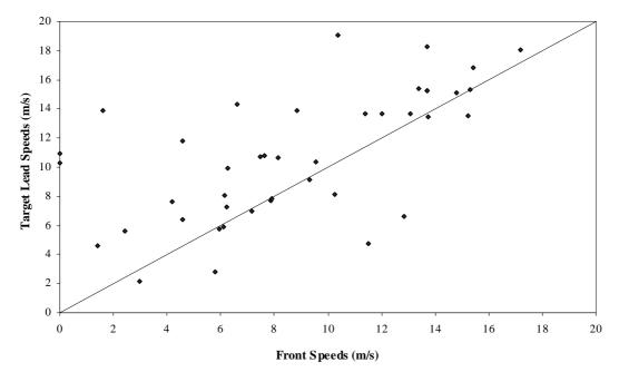
Figure 5 – Front and target lead speeds at the start of the lane changing event.
