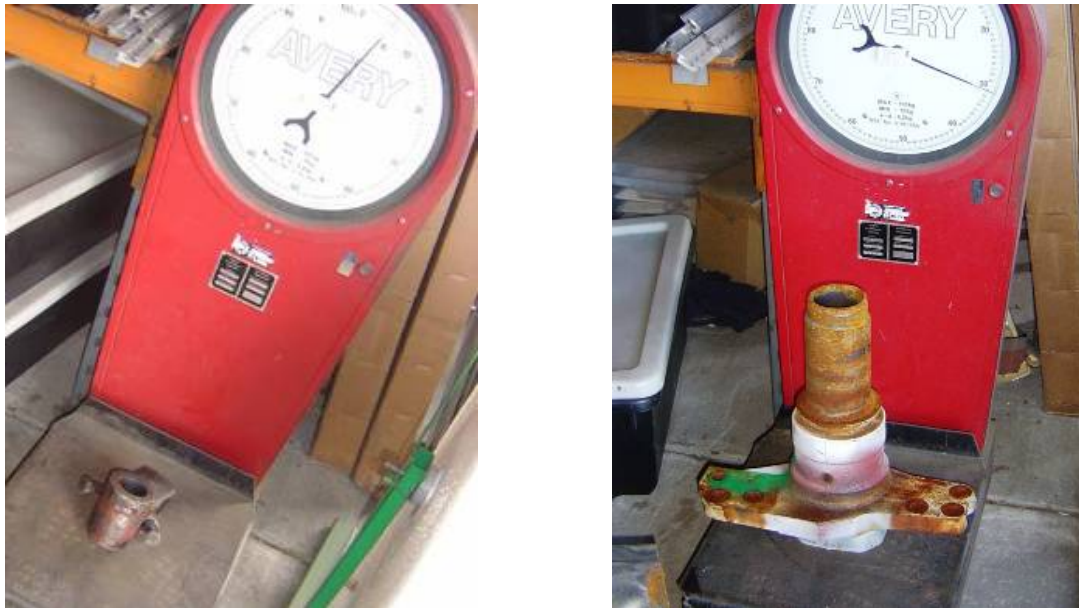
Figure 12 – Weighing the axle mass outboard of the strain gauges for the tag axle (left) and the drive axle (right)
