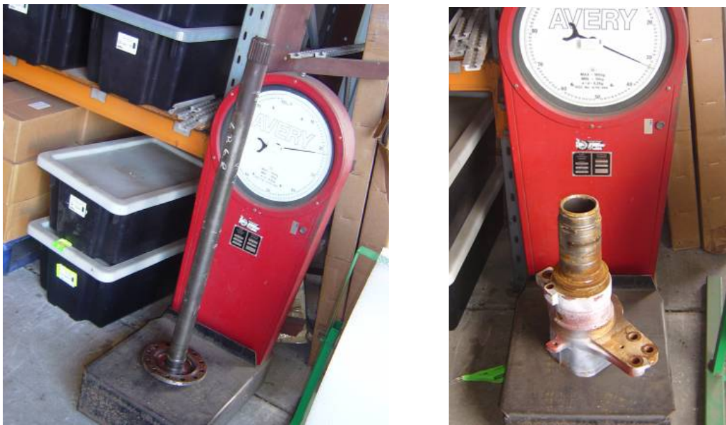
Figure 11 – Weighing the half-shaft mass outboard of strain gauges (left) and mass of bus drive axles outboard of strain gauges (right)
