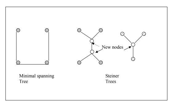
Figure 6: Minimal Spanning Tree and Steiner Tree
