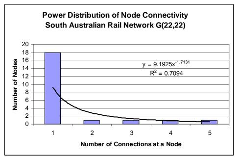
Figure 2: Nodal Connectivity of South Australian Rail Network
