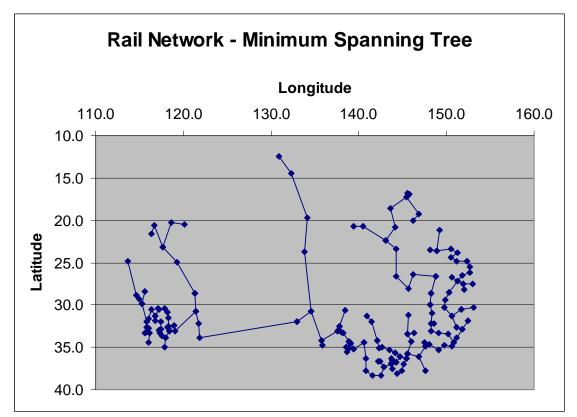
Figure 5: Minimal Spanning Tree of Australian Rail Network
