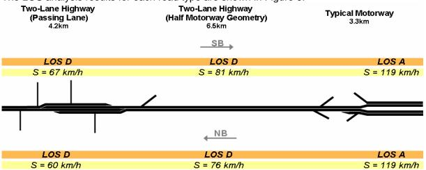
Figure 6: Results of HCM 2000 traffic operations analyses for the estimated peak hour
