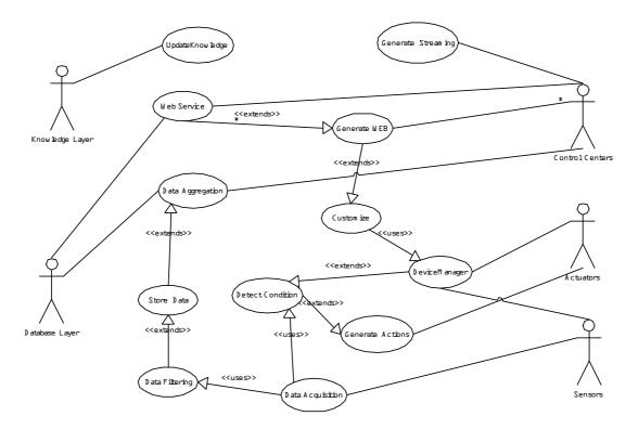
Figure 3. Use-case diagram of the front-end component
