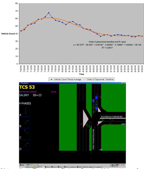
Figure 2 Intersection traffic volume profile (mean five min vehicle count over a four month period) at the intersection TS 53 (Port Wakefield Rd/Waterloo Corner Rd) extracted from ACTS VS data file and the intersection diagram from SCATS. The chart also graphs the polynomial trend line curve (red/smooth line).
