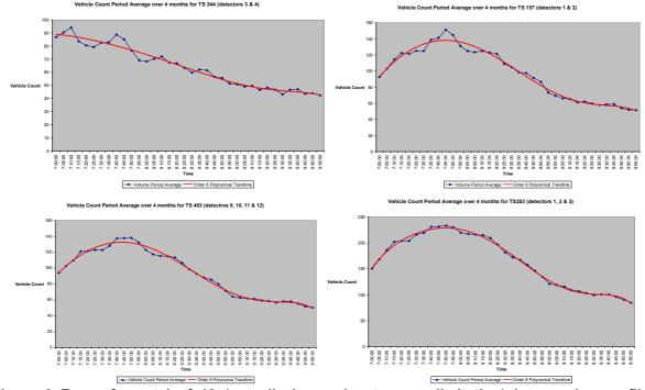
Figure 3 Four of a total of 12 (not all shown due to page limitation) intersection profiles comprising the southbound morning peak route along Port Wakefield Rd/Main North Road in the northern suburbs of Adelaide, in order of intersection heading from North to South: analysis of the pilot data investigation.
