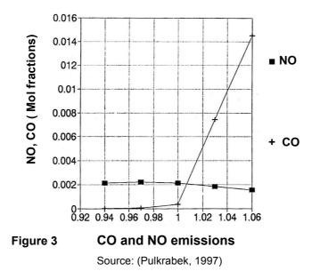
A change in one variable that reduces normally one emission may increase one or more other emissions (Schäfer and Basshuysen, 1995). CO depends almost exclusively on the air/fuel ratio, whereas  $NO_X$  and HC depend on several other influences, such as the chamber area, cylinder displacement, and ignition timing.
