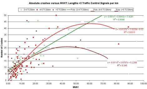
Figure 5 Absolute crashes versus MVKT for segments with more than 3 traffic control signals per kilometre
