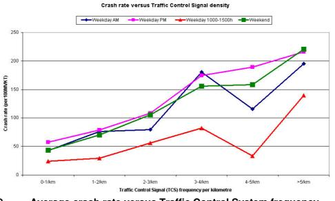
Figure 9 Average crash rate versus Traffic Control System frequency.
