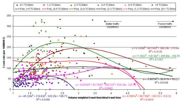
Figure 8 Crash rate (per 100MVKT) versus the traffic flow parameter P (volume weighted travel time/ideal travel time).
