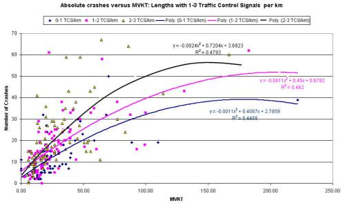
Figure 4 Absolute crashes versus MVKT for segments with 0-3 traffic control signals per kilometre
