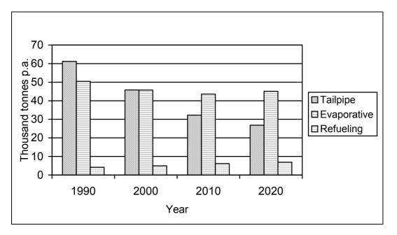
Figure 4: VOC emissions from passenger vehicles in Sydney
