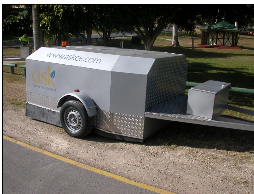
Figure 2 'Road Ear' Test Rig – for CPX Testing.
