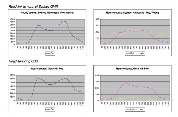
Figure 3 Car and heavy vehicle hourly counts (Classified Vehicle Counts Study)
