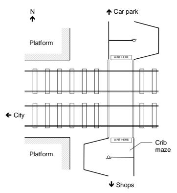
Figure 3: Layout of the trial crossing
