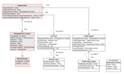
Figure 4 A sample class-object diagram for the car park/traffic signal objects
